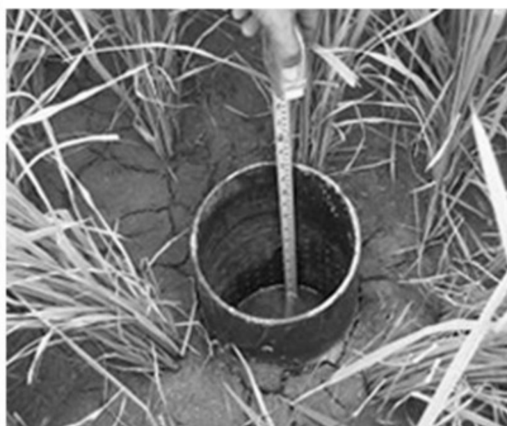
Fig 1: Field water tube as a simple tool to implement safe AWD (Bouman et al. , 2007 and Rice Knowledge Bank, IRRI)
